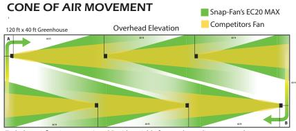
Turbulent airflow in corners A and B with variable factors depending on greenhouse structure Test conducted using hand held anemometers for informational purposes at BESS labs C18258 & C18279
