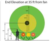
Snap-Fan EC20 MAX can match performance of Schaefer VK20 while using 25% less energy. Snap-Fan 265 watts at 3,870 CFM to VK20 351 watts for 3,870 CFM.
