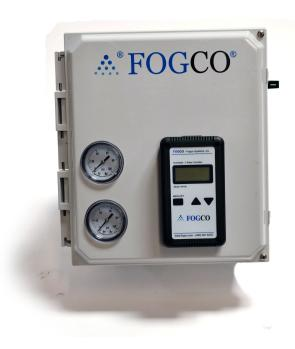
This Air Injection System Control Box is used to monitor and control the air injection system. It utilizes 230V power and plugs into any standard 15-amp receptacle. Water and air are fed into the box using ½" low pressure tubing. The output is automatically controlled by electric solenoid valves and adjustable pressure regulators.
