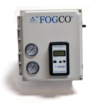
This Air Injection System Control Box is used to monitor and control the air injection system. It utilizes 115V power and plugs into any standard 15-amp receptacle. Water and air are fed into the box using ½" low pressure tubing. The output is automatically controlled by electric solenoid valves and adjustable pressure regulators.
