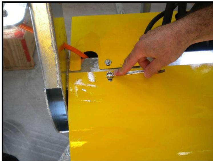
Remove the front protection and switch off the main switch (white arrow)
