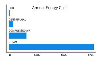
Analysis for moisture output of 1 GPM (500 pounds per hour) 10 hours per day, 365 days per year with a kW rate of \$.13 per hour
