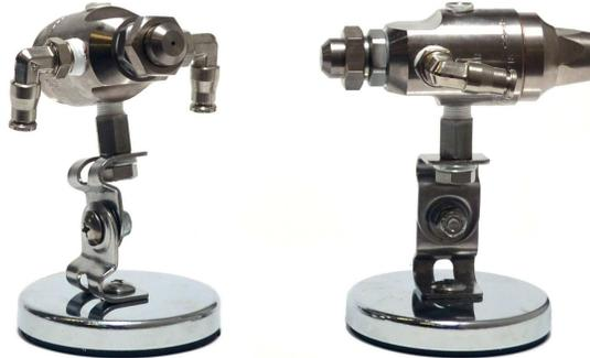
These Drip Free Fogco air injection nozzles are all stainless steel and rated for use with treated and aggressive water. They are mounted on a magnetic base for quick and simple installation and provide both vertical and horizontal adjustment of the direction of the fog.
