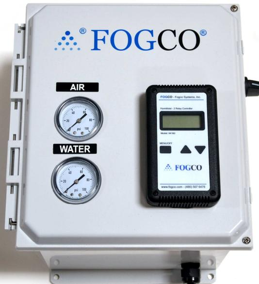
This Air Injection System Control Box is used to monitor and control the air injection system. It requires 80 psi air pressure, 25 cfm air supply, and 60 psi water pressure to provide maximum performance. It utilizes 115V power and plugs into any standard 15 amp receptacle. Water and air are fed into the box using ½” low pressure tubing. The output is automatically controlled by electric solenoid valves and adjustable pressure regulators.
